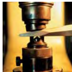
Special tool control for blade hardness.
